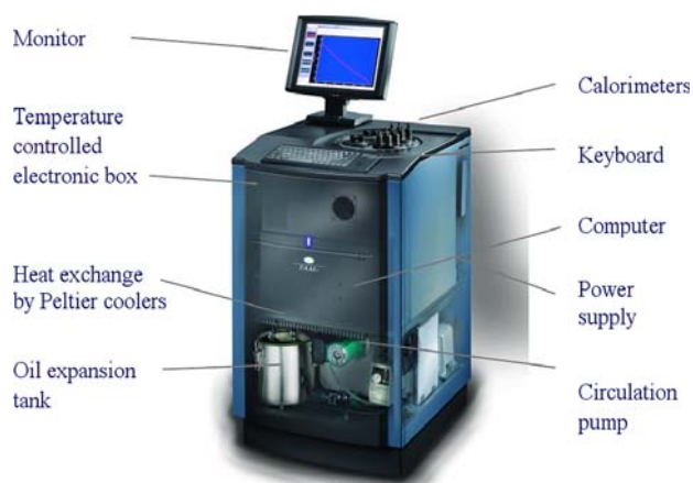
Fig. 1 Structure of TAM III [9]
